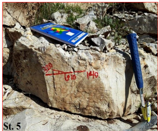
Fig. (33): Fault-slip data analyses for 4 dextral strike slip faults with field photo in the station 5. The paleostress are:
