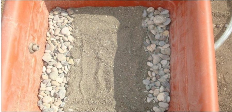
Plate (7): Constructed wetland horizontal subsurface flow
