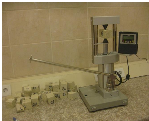
Fig. 8 Point load test
