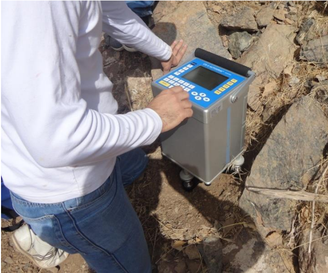
Figure -5: Data acquisition using Scintrex CG-5 gravimeter in the field
