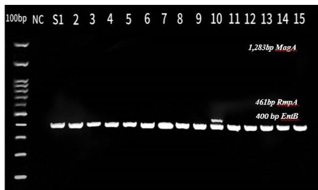
Figure 3. Multiplex PCR for magA , rmpA and entB for K. pneumoniae 100 bp DNA ladder NC: Negative Lane 1-15 is positive for entB , negative for magA , and only sample 10 is positive for rmpA .
